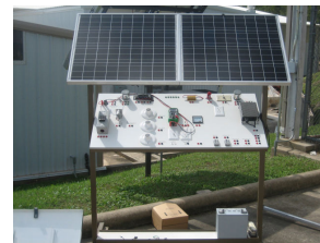
FIG. 7 MINI-LABORATORY EDUCATIONAL FOR EXPERIMENTAL STUDIES TO THE CONCEPT OF RENEWABLE ENERGY
